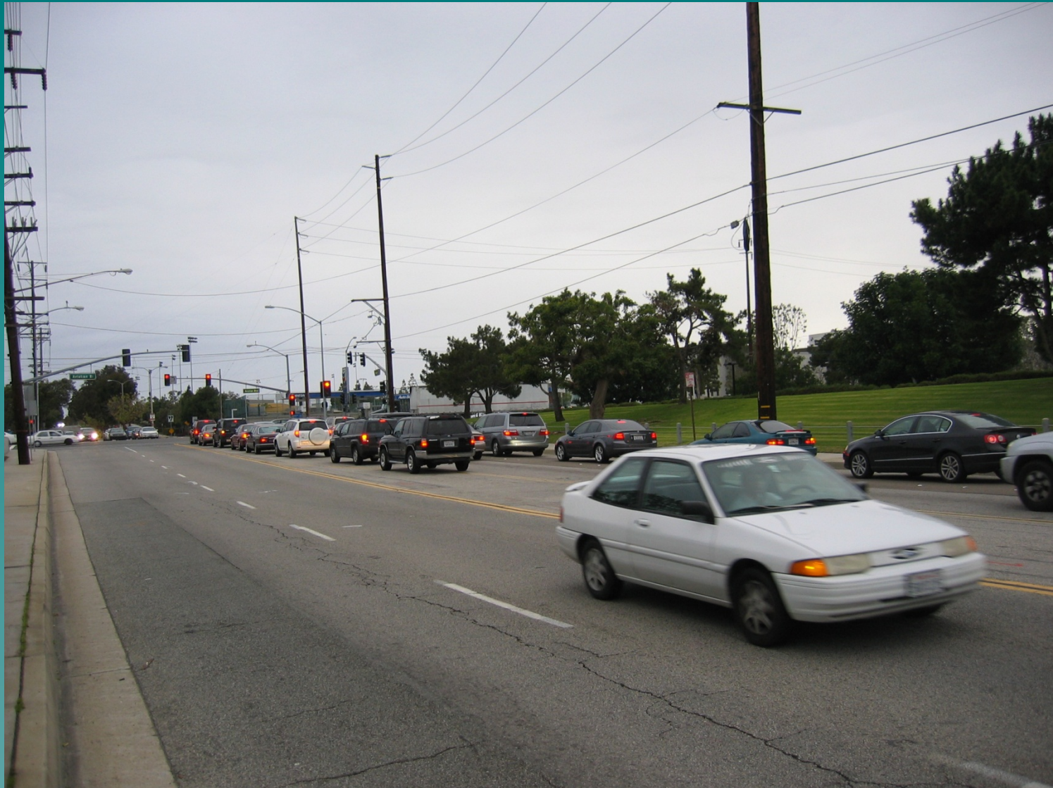
Marine Ave.- East of Aviation intersection. WB through lane congested due to heavy WB right-turn movement.
