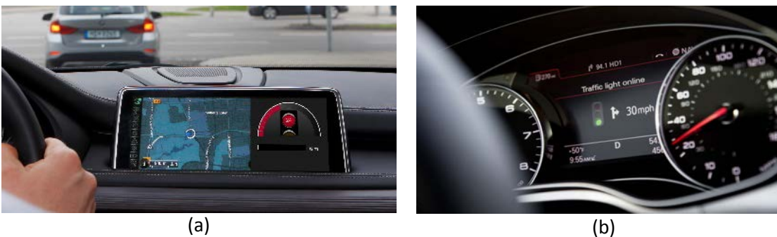
Figure 2. Examples of in-vehicle human machine interface (HMI) designs that present traffic signal data to drivers: (a) red countdown dial or speed advice together with navigation display in the central control (BMW) (b) red countdown timer or speed advice on digitalized dashboard (Audi).
