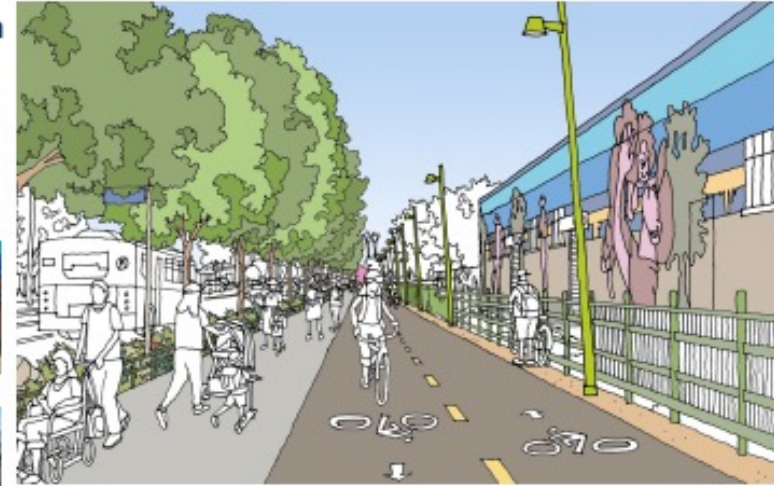
View looking West | Note: 2' painted buffers will be provided between walk and bike path and adjacent uses
