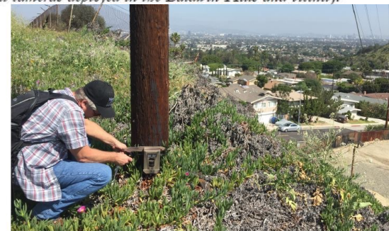
Figure 5-2. Typical camera top deployment at optimal height (approx. 30 cm) for activation by medium-sized mammals.
