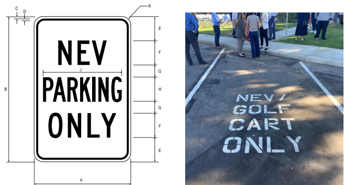
Figure 19. NEV parking sign, marking, and charging options
