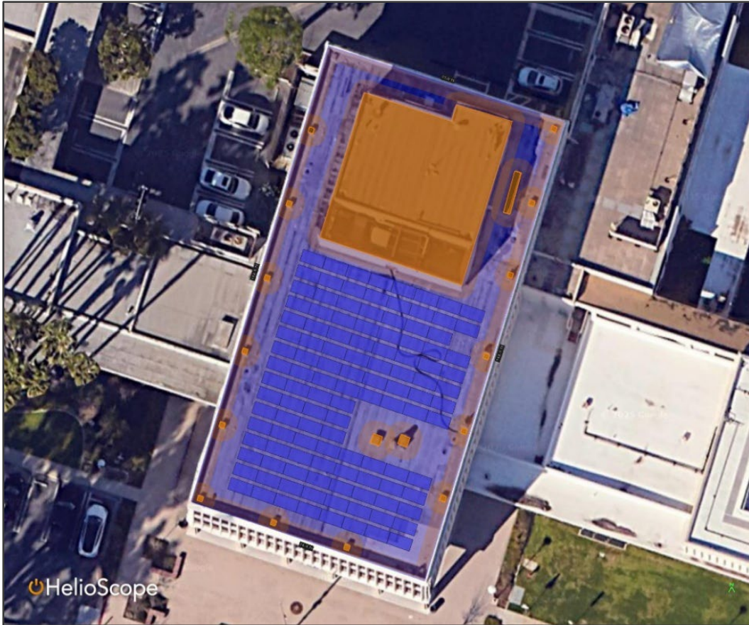
Figure 36 Proposed Solar PV – Torrance City Hall
